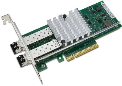
Intel X520 10 GbE Dual SFP+ SR Ethernet Converged Network Adapter
