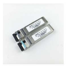
FiberHome 10G SFP+ BIDI Tx-1270nm RX-1330nm 40km Transceiver-Modul
