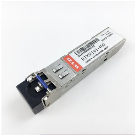
WTD 1250M 1310nm SM 10km ESFP SFP-Transceiver-Modul
