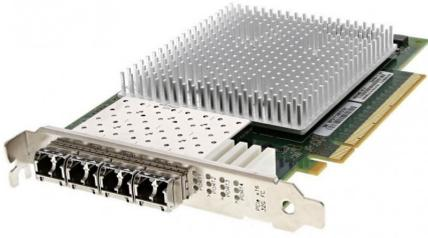
Original Qlogic QLE2764-SR-CK PCIe 3.0 x16 Quad-Port 32GFC SR-Optic SFP+ 32Gb Fibre Channel Adapter
