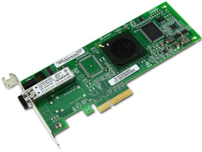
Original Qlogic QLE2460-CK PCI Express x4 Single-Port 4 Gb Fibre Channel Host Bus Adapter
