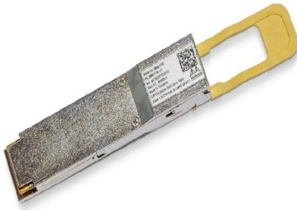
Mellanox MMA1T00-VS 200GBASE-SR4 QSFP56 850nm 100m DOM MTP/MPO-12 MMF Optisches Transceiver-Modul
