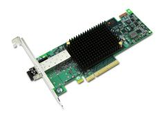
Emulex LPe16000 Gen 5 16GFC PCIe 3.0 Single-Port Fibre Channel Host Bus Adapter
