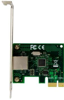
Intel I210 Single RJ45 Port Ethernet Server Adapter, 10/100/1000, PCIe v2.1 (2,5 GT/s) x1
