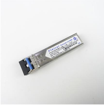
II-VI Finisar Optischer Transceiver, eSFP, 1310 nm, 2,67 Gbit/s, -9,5~-3 dBm, -18,0 dBm, LC, SM, 2 km
