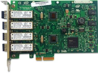
Intel PRO/1000 PF Quad-Port-Serveradapter, LC, 1000BASE-SX Multimode, PCIe, 82571 GB
