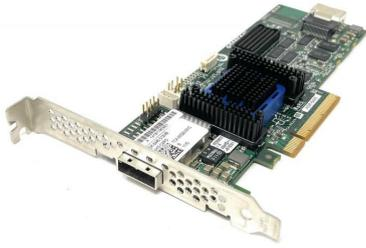
Adaptec ASR-6445 2270200-R 6 Gb/s 8-Port (4 intern/4 extern) PCIe Gen 2 x8 SAS SATA RAID Controller
