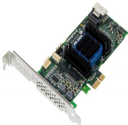
Adaptec ASR-6405E 2270800-R 6 Gb/s PCIe Gen2 x1 4-Port Int.SAS/SATA RAID Controller
