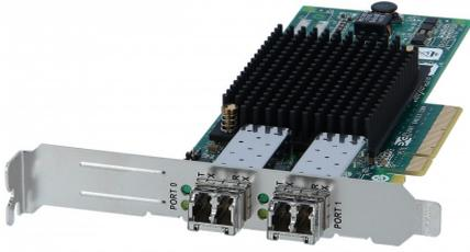
HPE 82E 8 GB 2-PORT PCIe x8 FIBER CHANNEL HOST BUS ADAPTER, 697890-001
