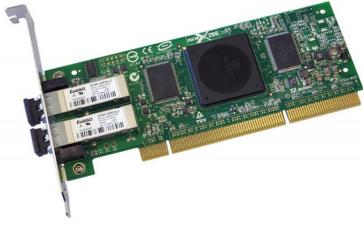
HPE 4 GB 2-PORT PCI-X 2.0 FIBRE CHANNEL HOST BUS ADAPTER, AB379-60101
