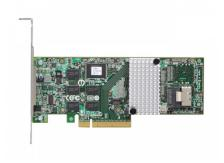
Broadcom 3ware 9750-4i LSI00215 PCIe 2.0 x8 4-Port Internal 6 Gb/s SATA+SAS RAID Controller Card 9750-4i
