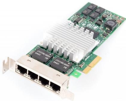
HPE NC364T PCI-E QUAD PORT GIGABIT SERVER ADAPTER, 436431-001, 435506-003
