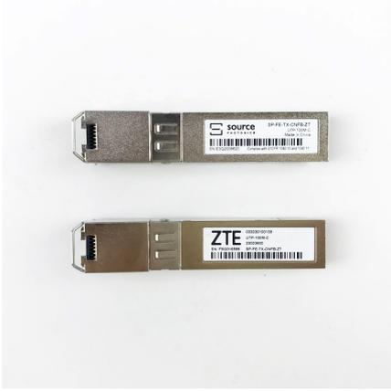
ZTE 100M UTP 100m C-temp Kupfer SFP SP-FE-TX-CNFB-ZT EOLT-C03-02-E
