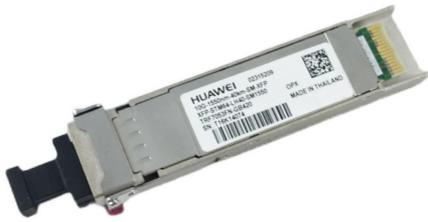
Huawei XFP-STM64-LH40-SM1550 Optischer Transceiver, XFP, 10G, Singlemode-Modul (1550 nm, 40 km, LC)
